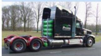
Demo truck with LPG, CNG and LNG tank package
